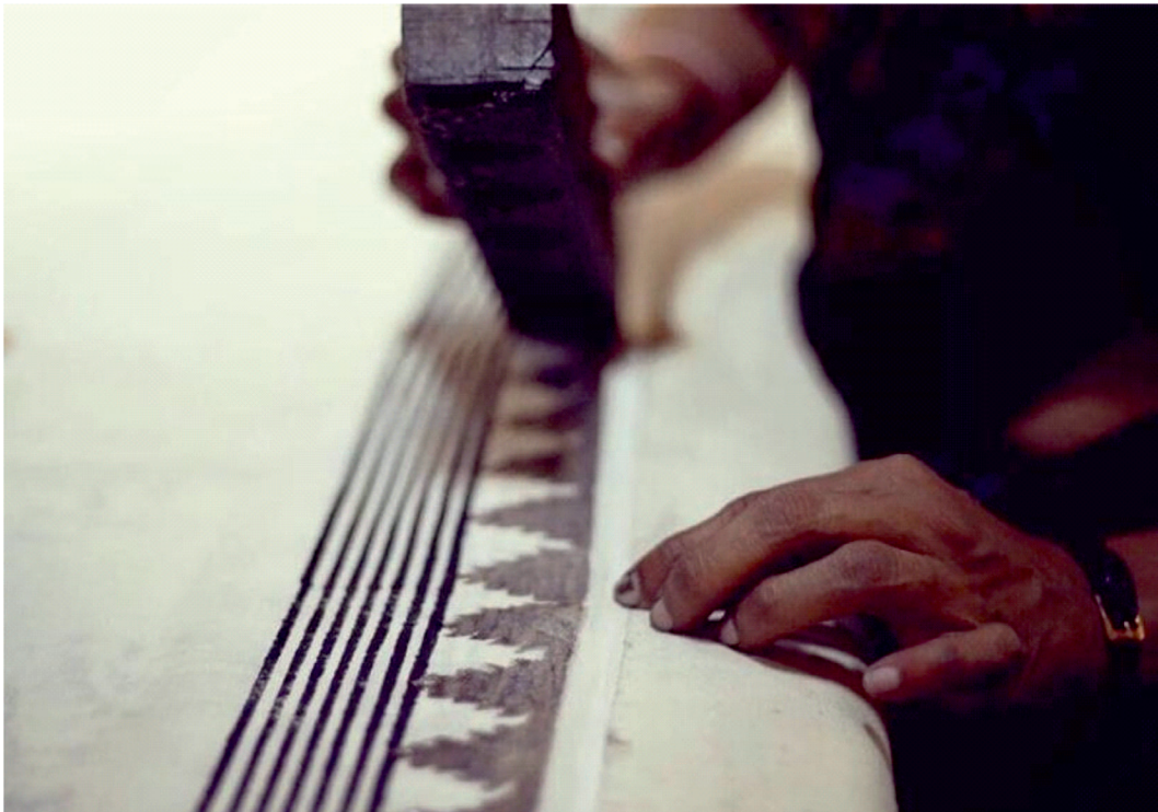
[Fig 1.3] A worker at Charaka carefully creating block-print patterns onto fabrics using a wooden hand-block.
